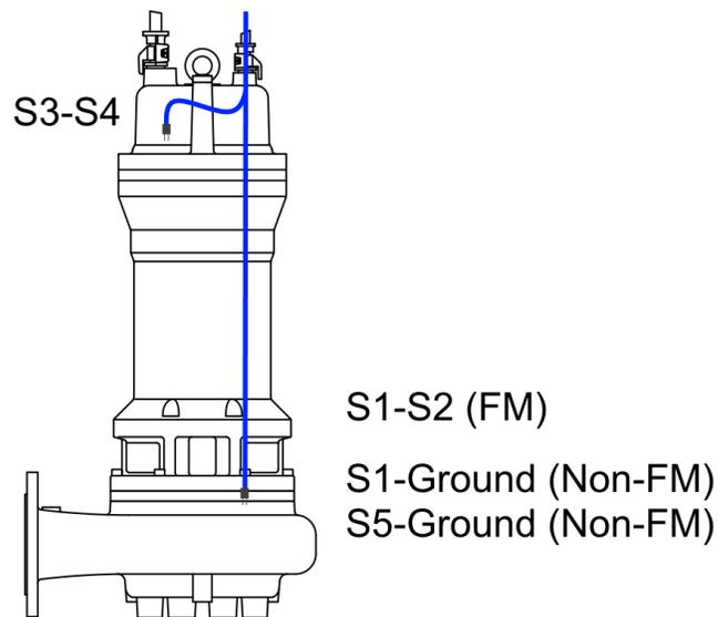
If the pump is equipped with an optional dual wire motor chamber seal monitor, it will be wired as S5 & S6.
