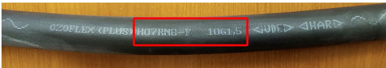
Cable size is printed on the cable above as “**10G1.5.**” This means this cable has Qty.10 leads that are 1.5 sq mm in cross-section. H07RN cable sizes are given as (# of conductors) G (size of conductors in sq.mm). E.G., 4G4, 5G1.5, 7G1.5
