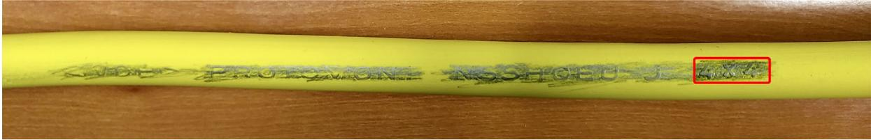
Cable size is embossed on the cable above as “4x4.” This means this cable has Qty.4 leads that are 4 sq mm in cross-section. NSSHOU cable sizes are given as (# of conductors) x (size of conductors in sq.mm). E.G., 4x1.5, 7x2.5, 4x25
