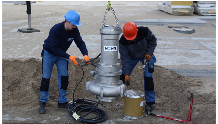
For chemically aggressive liquids: Stainless steel submersible pumps.
